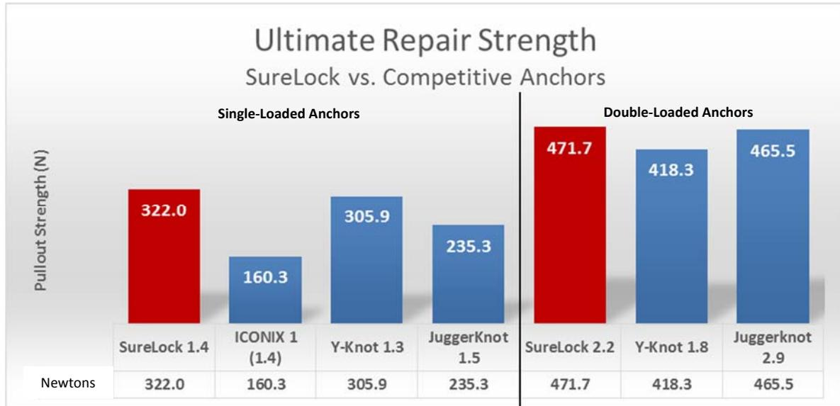
**TABLE 1.** SureLock and competitive anchor mean load to failure (N).
